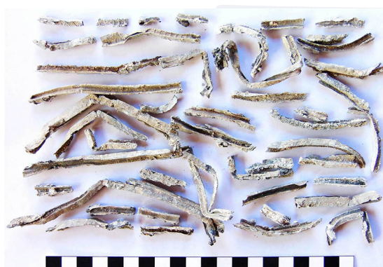
Figure 16: H-section lead comes (in which the cut glass pieces were inlaid), Dubrovnik cathedral, 14th–15th century.
