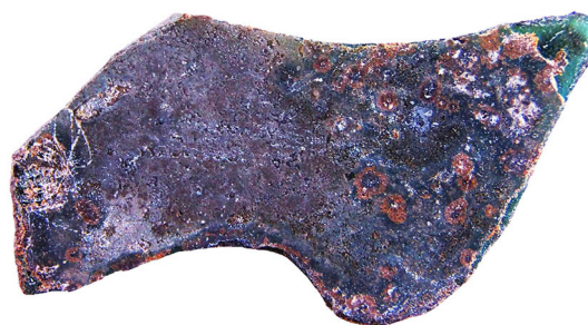
Figure 18: Corrosion on a piece of green stained glass (H. 35 cm, W. 7.5 cm), Dubrovnik cathedral, 14th- 15th century.
